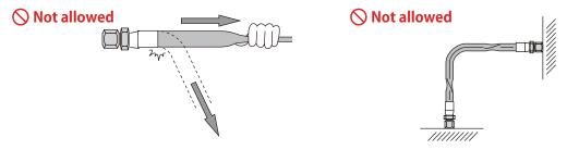
4. Protect TOYOX hose assemblies from external damage. If TOYOX hose assemblies contact other objects (machines, equipment, etc.), the hose could rupture from external damage, or the coupling could be damaged.
